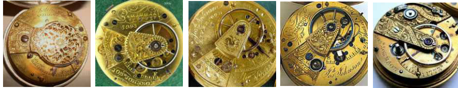
A Full-width pierced table B Double wedge, cutaway foot C Double wedge, full-length foot D Single wedge, cutaway foot E Parallel-sided
